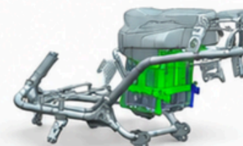
Improved Supporting Structure (CAD Model)
